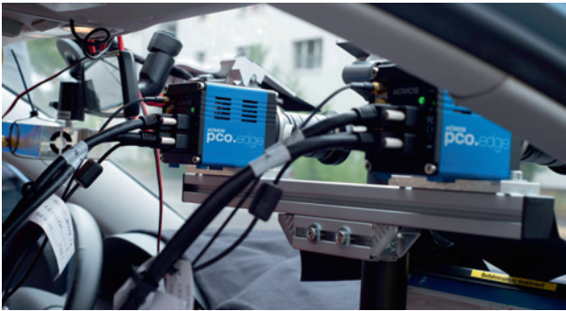
Figure 5: Reference stereo set-up with two pco.edge 5.5 cameras to acquire ground truth for driver assistance systems with 960 \times 2560 pixel at 200 fps.
