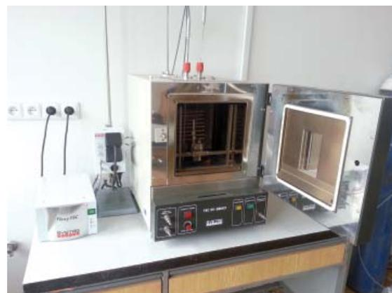
Fig. 2 Safety calorimeter SEDEX
