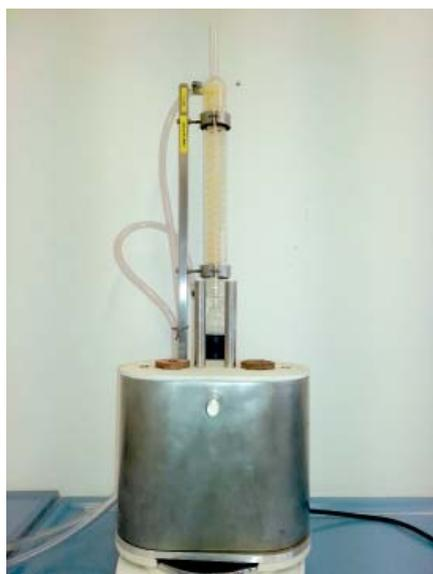
Fig. 1 Device for Differential Mackey Test
