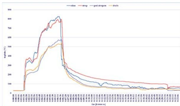
Fig. 8 The temperature for all thermocouples during the test no. 4
