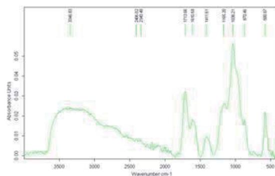
Fig. 1 FT-IR spectrum of the foil GO- Biochar
