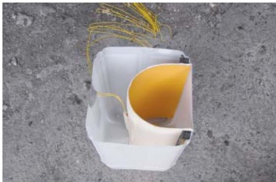
Fig. 6 and 7 Produced charges in two sizes and with placed explosive
