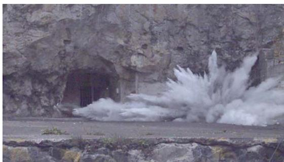
Fig. 8 and 9 Test of an improvised water charge 5 l,  $t = 0.6 \text{ ms}$  and 10 l,  $t = 1.5 \text{ ms}$
