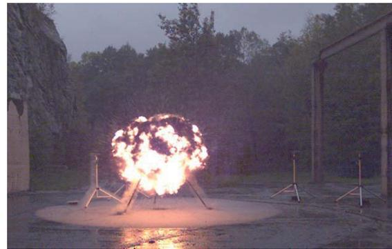
Fig. 2 Test of the uniformity of explosion of the Semtex 10-SE explosive,  $t = 5,236 \text{ ms}$
