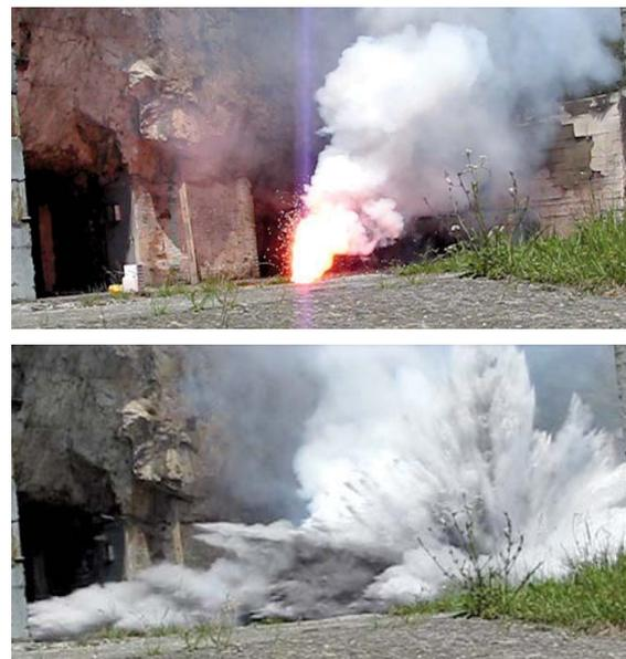
Fig. 13 Practical test of water spout when extinguishing the flame created by using 20 pcs of PS-25
