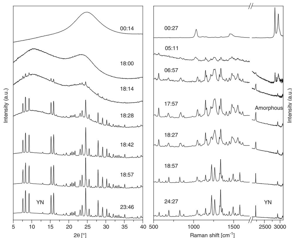
**Fig. 2:** *In situ* X-ray diffraction pattern (left) and Raman spectra (right) recorded during the crystallization of ROY from a solution in methanol using an acoustic levitator as a sample holder. The evaporation of the solvent leads to the formation of an amorphous phase which crystallizes to the YN polymorph.
