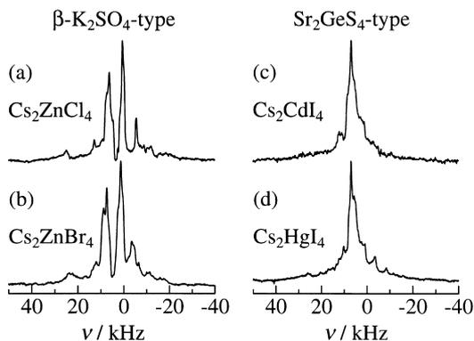
Fig. 1. Quadrupolar perturbed  $^{133}\text{Cs}$  NMR spectra at 39.4 MHz at room temperature in  $\text{Cs}_2\text{ZnCl}_4$  (a) and  $\text{Cs}_2\text{ZnBr}_4$  (b) with  $\beta\text{-K}_2\text{SO}_4$  structure, and  $\text{Cs}_2\text{CdI}_4$  (c) and  $\text{Cs}_2\text{HgI}_4$  (d) with  $\text{Sr}_2\text{GeS}_4$  structure.
