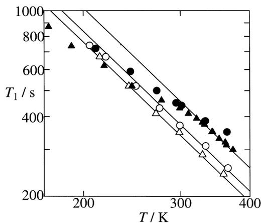
Fig. 3. Temperature dependences of  $^{133}\text{Cs}$  NMR  $T_1$  in  $\text{Cs}_2\text{ZnCl}_4$  (●) and  $\text{Cs}_2\text{ZnBr}_4$  (▲) with  $\beta\text{-K}_2\text{SO}_4$  structure, and  $\text{Cs}_2\text{CdI}_4$  (○) and  $\text{Cs}_2\text{HgI}_4$  (△) with  $\text{Sr}_2\text{GeS}_4$  structure. Solid lines are theoretical curves calculated by using (3).
