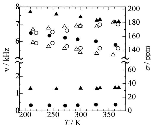
Fig. 2. Temperature dependences of central peak frequencies  $\nu$  and their chemical shifts  $\sigma$  in  $^{133}\text{Cs}$  NMR spectra for  $\text{Cs}_2\text{ZnCl}_4$  (●) and  $\text{Cs}_2\text{ZnBr}_4$  (▲) with  $\beta\text{-K}_2\text{SO}_4$  structure, and  $\text{Cs}_2\text{CdI}_4$  (○) and  $\text{Cs}_2\text{HgI}_4$  (△) with  $\text{Sr}_2\text{GeS}_4$  structure.
