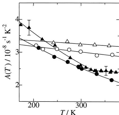
Fig. 4. Temperature dependences of  $A(T)$  values in (3) obtained by substitution of  $^{133}\text{Cs}$  NMR  $T_1$  for  $\text{Cs}_2\text{ZnCl}_4$  (●) and  $\text{Cs}_2\text{ZnBr}_4$  (▲) with  $\beta\text{-K}_2\text{SO}_4$  structure, and  $\text{Cs}_2\text{CdI}_4$  (○) and  $\text{Cs}_2\text{HgI}_4$  (△) with  $\text{Sr}_2\text{GeS}_4$  structure. Solid lines are fitting curves assumed exponentially temperature dependent functions.
