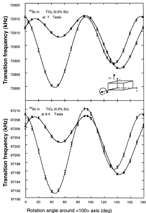
Fig. 1. FT-NMR of  $^{45}\text{Sc}$  at  $H = 7.0$  T and 9.4 T. Resonance frequencies of  $^{45}\text{Sc}$  as a function of crystal orientation. The crystal was rotated around the axis placed almost parallel to  $\langle 100 \rangle$  which was perpendicular to  $H_0$ . The  $m = \pm 1/2 \leftrightarrow \mp 1/2$  transition frequencies were observed under the external fields of 7.0 T and 9.4 T.
