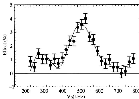
Fig. 2. Quadrupole spectrum of  $^{41}\text{Sc}$  implanted in  $\text{TiO}_2$  at high field. The asymmetry change was measured as a function of the quadrupole coupling frequency,  $\nu_Q = 3eqQ/2I(2I - 1)$ . The solid curve is the best fit of the theoretical curve to the data.
