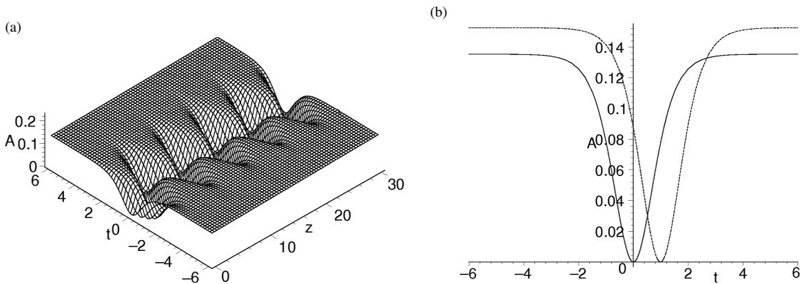
Fig. 3. (a) Travelling solitary wave solutions with chirp, as functions of the propagation distance. Intensity  $|\psi|^2$  of solution 1 from Table 1. Coefficients and parameters:  $\beta(z) = \cos z$ ,  $g = 0.04$ ,  $M = 1$ ,  $a_0 = 0.001$ ,  $f_{10} = 1$ ,  $k_0 = 1$ ,  $l_0 = 0$ ,  $\beta_0 = 1$ ,  $k_b = 1$ , and  $b_0 = 1$ ; (b)  $z = 0$  (solid),  $z = 30$  (dash).
