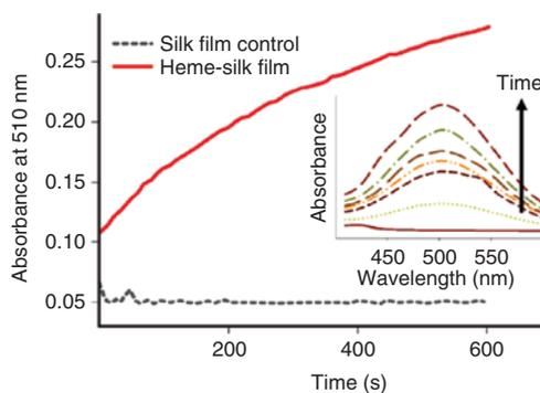
**Figure 8:** Catalytic activity of a heme *b*-AmelF3 film. Coupling of phenol to 4 amino-antipyrene gives a coloured quinone. The inset shows the change in the solution UV/vis spectrum over time. Reprinted and adapted from [100] under Creative Common Licence.
