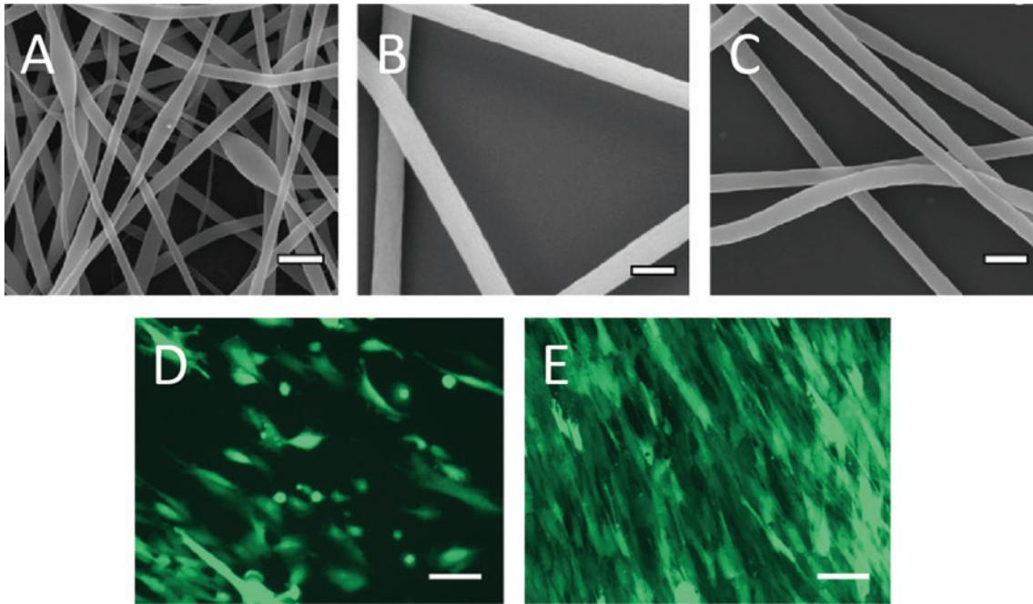
**Figure 5:** Electrospun fibres made of recombinant honeybee silk and cells cultured on mats made thereof. (A)–(C) Scanning electron microscopy (SEM) images of fibres from 12.5% AmelF3 protein solutions complemented with (A) 0.4%, (B) 0.67%, and (C) 1% PEO. Scale bars: 500 nm. (D)–(E) Fluorescent images of GFP-expressing fibroblasts grown on electrospun fibre mats for (D) 1 day and (E) 7 days. Scale bars: 100  $\mu\text{m}$ . Reprinted and adapted with permission from [78].
