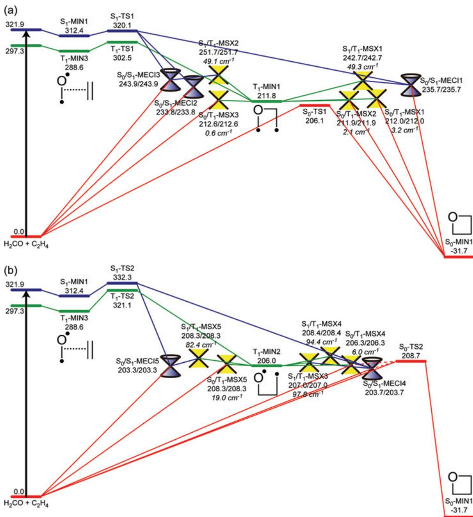
**Fig. 2.** Potential profiles for (a) the C-O-C-C biradical path and (b) the O-C-C-C biradical path, based on the energetics of CASPT2[6e, 50]/AVDZ (in kJ/mol) in Fig. 1. At MSX structures, spin-orbit coupling values are shown in italic in cm<sup>-1</sup>.
