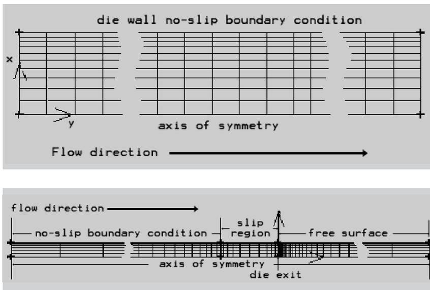
Figure 4 (left above): Mesh design for a) stress relaxation simulation and b) extrudate swell simulation.
