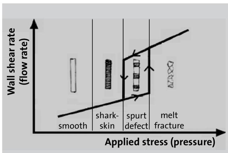
Figure 1: Typical flow curve of polymer melts and general extrudate classifications.
