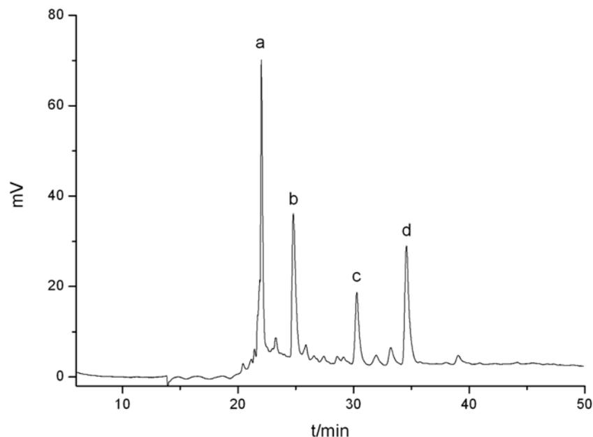
**Fig. 9** RP-HPLC profile of crude heptapeptide **1** with serious racemization (**a**  $t_R$  22.02 min, **b**  $t_R$  24.78 min, **c**  $t_R$  30.27 min, **d**  $t_R$  34.58 min ). According to the  $t_R$  24.80 min of heptapeptide **1** in Fig. 2, **b** was the desired heptapeptide **1**, and **a**, **c** and **d** were its diastereoisomers.
