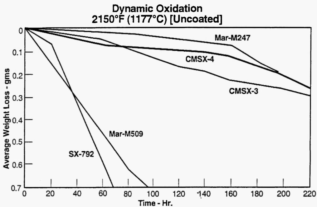
Fig. 4: Oxidation resistance of CMSX-4 compared to other alloys.
