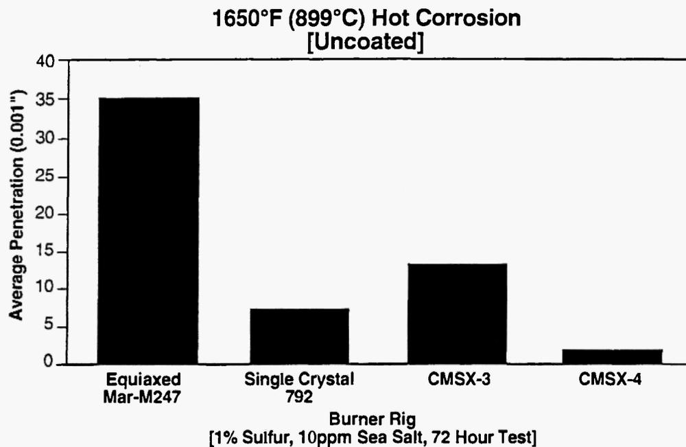
Fig. 5: Hot corrosion resistance of CMSX-4 compared to other alloys.
