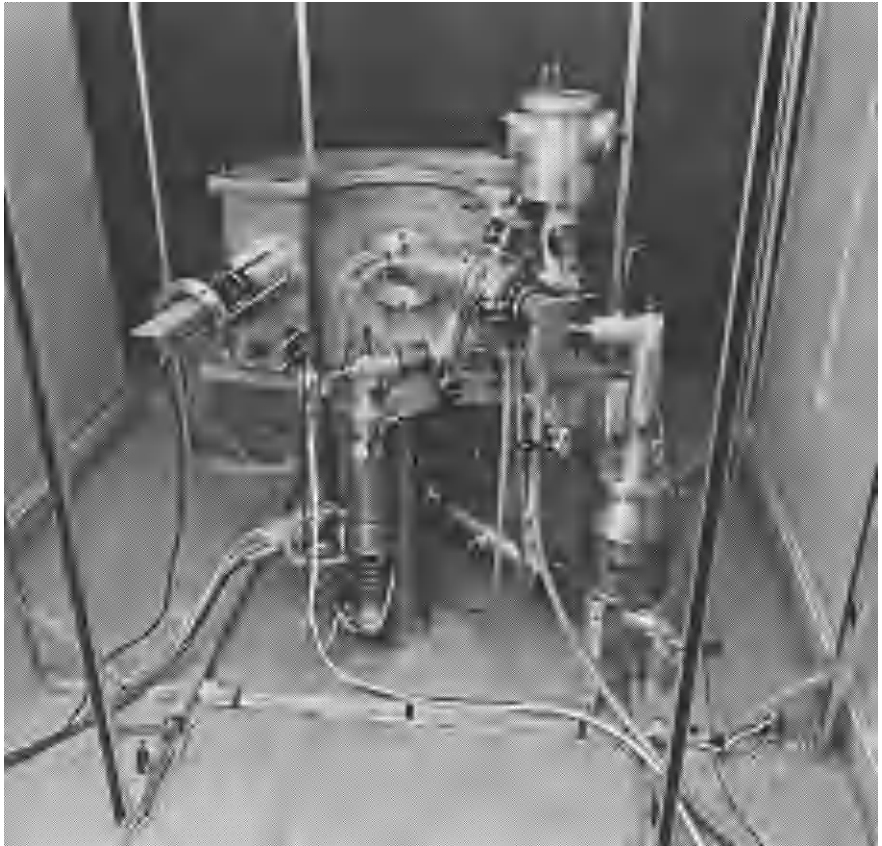
Fig. 5. Photograph of the prototype ESCA instrument according to Fig. 4. For further developments see Fig. 42.
