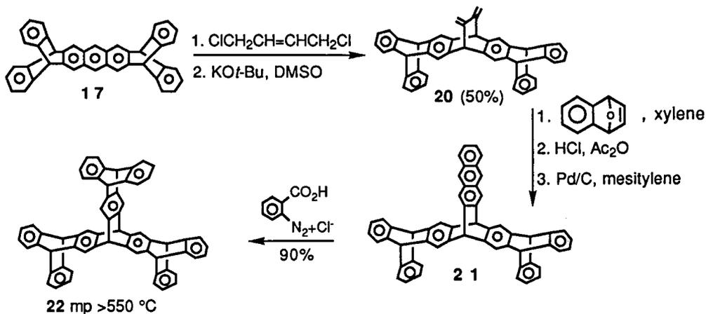
Noniptycene **22** has the molecular formula  $\text{C}_{62}\text{H}_{38}$ , but the  $D_{3h}$  symmetry reduces the NMR spectra to just 8 unique carbon and 5 unique proton signals.
