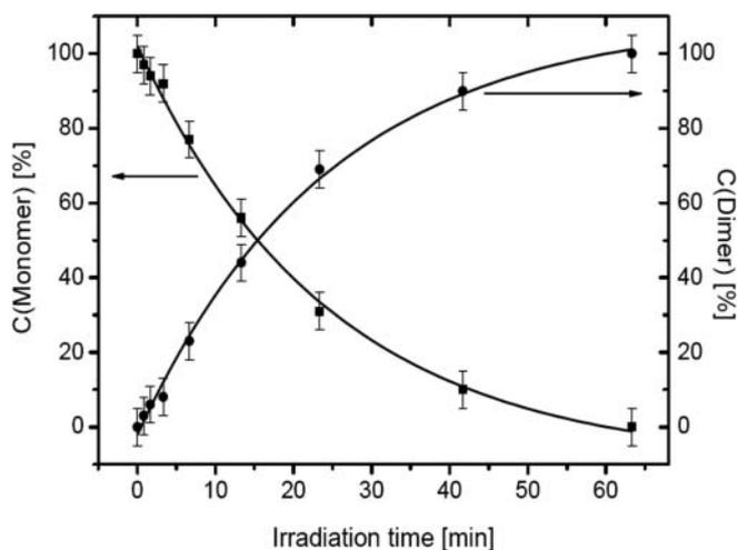
**Fig. 5.** [2 + 2] cycloaddition reaction of 2-benzyl-5-benzylidene-cyclopentanone. The conversion rate, based on refinements against single-crystal data, from the monomer to the dimer state is shown as changes in molar fraction  $C$  as a function of irradiation time.
