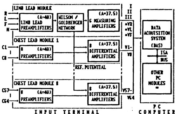
Fig. 1. Block diagram of the CardioPC mapping system.
