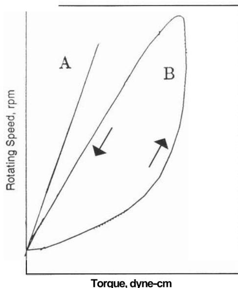
*Fig. 1. Typical rheological test in the mill. Shear rate is increased in time and then decreased. Curve A represents a Newtonian fluid. Curve B is a thixotropic fluid*
