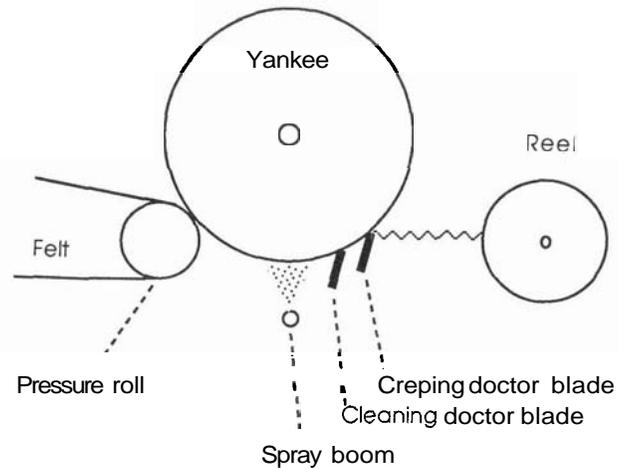
*Fig. 1. Schematic of tissue machine dry end.*
