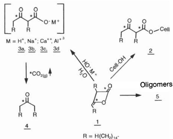
Fig. 1. Possible AKD reaction products produced during the sizing of paper.
