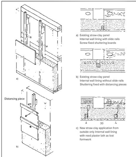
Fig. 201 Internal wall lining for renovation of a half-timbered structure
