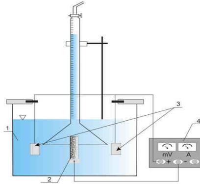
Fig. 2. The system of electrolytic hydrogenation of tested materials: 1 - an aqueous solution of sulphuric(VI) acid with the addition of 2 mg/dm<sup>3</sup> As<sub>2</sub>O<sub>3</sub>, 2 - tested material, 3 - platinum electrodes, 4 - ammeter and voltmeter
