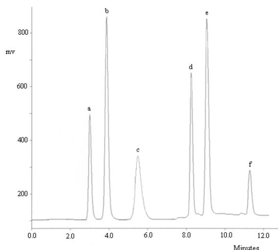
**Figure 3.** Representative chromatogram of quinapril, HCTZ and their degradation products: (a), DSA (b), HCTZ (c), quinaprilat (d), cloxacillin sodium (e), quinapril Hydrochloride (f), DKP: 1 mV: 0.001 AU.
