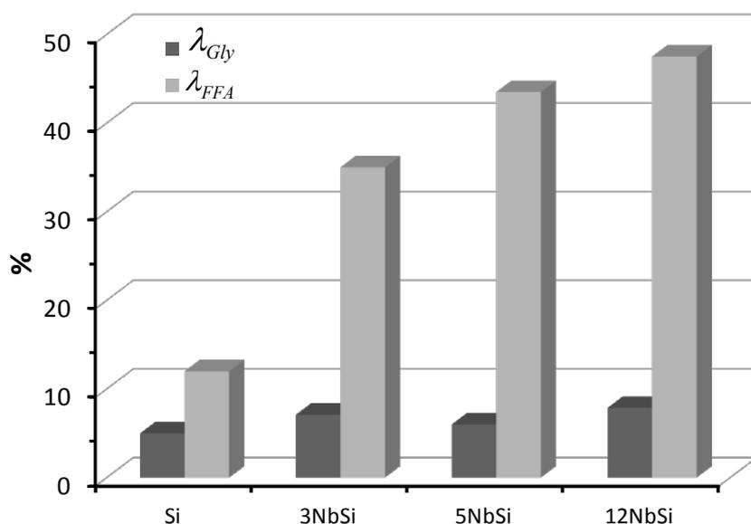
**Figure 1:** The conversion of triglycerides ( $IGly$ ) and FFA ( $IFFA$ ) of acid soybean oil (FFA =10% w/w) obtained with  $Nb_2O_5$  supported on silica catalysts. Reaction time = 1 h, reaction temperature = 180°C, catalyst = 0.1 g, acid soybean oil = 2 g, methanol =0.88 g.
