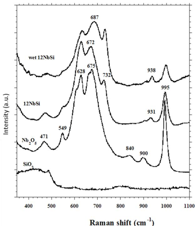
**Figure 5.** Raman spectra of the 12NbSi catalyst, at ambient condition and wet (wet12NbSi),  $\text{Nb}_2\text{O}_5$  and  $\text{SiO}_2$ .
