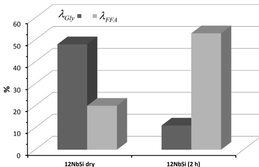
**Figure 6:** The conversion of glyceride groups ( $I_{\text{GLY}}$ ) and of FFA ( $I_{\text{FFA}}$ ) of acid soybean oil (FFA =  $10\%$  w/w) obtained with the 12NbSi catalyst. 12NbSi dry = dried at  $300^\circ\text{C}$ ; 12NbSi (2 h) = exposed to atmosphere for 2 h; (Reaction time = 1 h, reaction temperature =  $180^\circ\text{C}$ , catalyst = 0.1 g, acid soybean oil = 2 g, methanol = 0.88 g)
