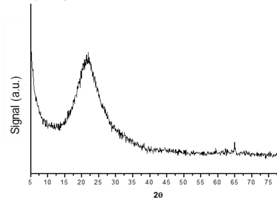
Figure 2: Powder XRD pattern of the 12NbSi catalyst.
