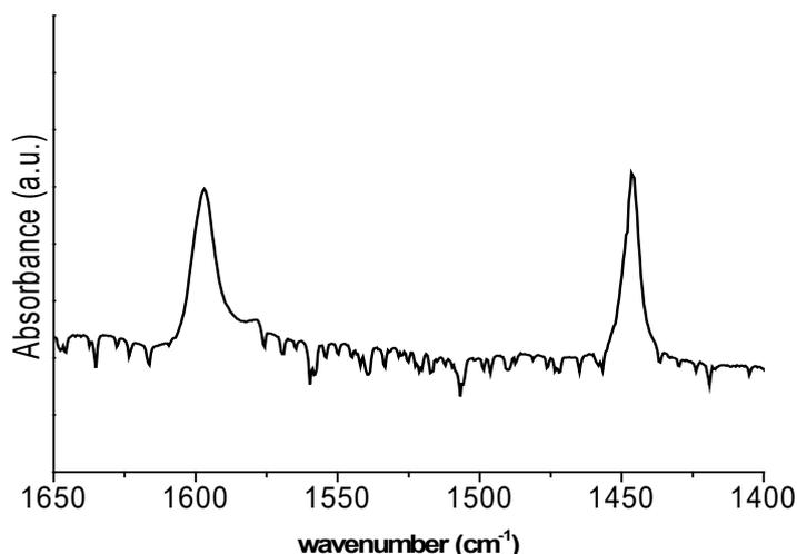
**Figure 4:** FTIR spectrum of adsorbed pyridine of the 12NbSi catalyst (pretreated at 300°C overnight under vacuum) at 25°C.
