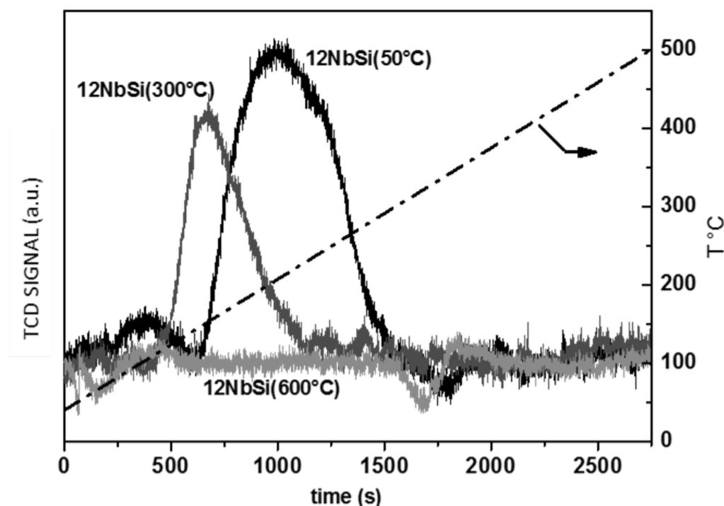
**Figure 3:** NH<sub>3</sub>-TPD profiles for the 12NbSi catalyst pretreated at 600°C, 300°C and 50°C.
