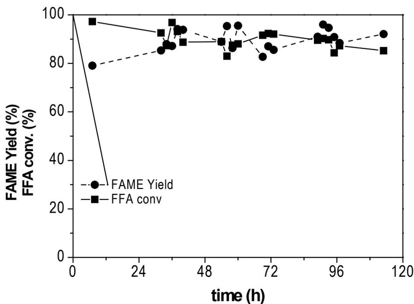
**Figure 7-** FFA conversion and FAME yield obtained in continuous run 1. Methanol 5.3 cm<sup>3</sup>/min; acid oil 2.6 cm<sup>3</sup>/min (FFA = 10 % w/w); T=220°C; Cat. 12NbSi.
