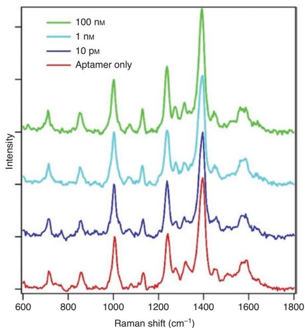
**Figure 2:** Normalized SERS spectra obtained from (red) only the aptamer, and the aptamer with (blue) 10  $\mu\text{M}$ , (light blue) 1  $\text{nM}$ , (green) 100  $\text{nM}$  MnSOD. Each spectrum is an averaged spectrum at 10 different places on the same substrate. A 660 nm CW laser (0.4 mW) was used for SERS excitation and the signal was acquired for 30 s for each spectrum. Background was removed and baseline was offset for clarity.
