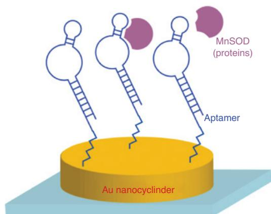
**Figure 1:** Schematic of the SERS sensor of MnSOD using a specific aptamer.
