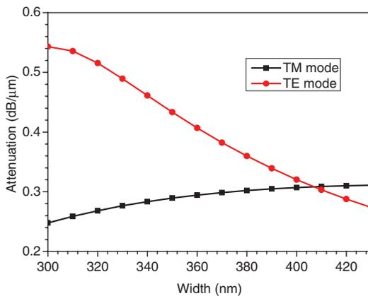
**Figure 3:** Attenuation versus graphene-Si waveguide width.
