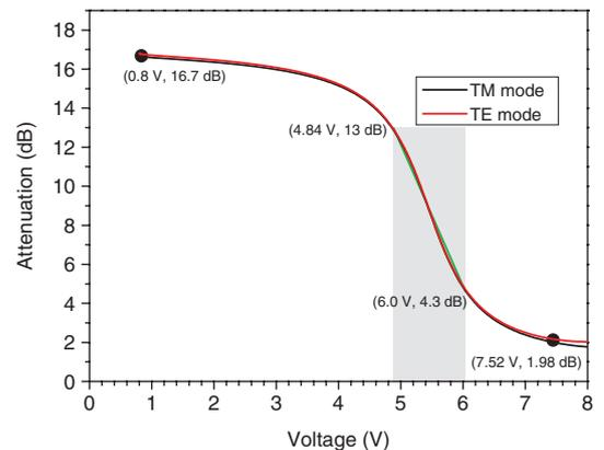
**Figure 7:** Attenuation of graphene-based polarization-insensitive optical modulator versus drive voltage.
