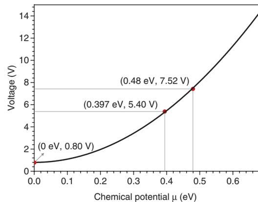
**Figure 6:** Drive voltage of the graphene-based polarization-insensitive optical modulator versus the chemical potential of graphene.
