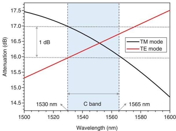
**Figure 5:** Attenuation of graphene-based polarization-insensitive optical modulator versus incident light wavelength for two supported TM and TE polarized modes.
