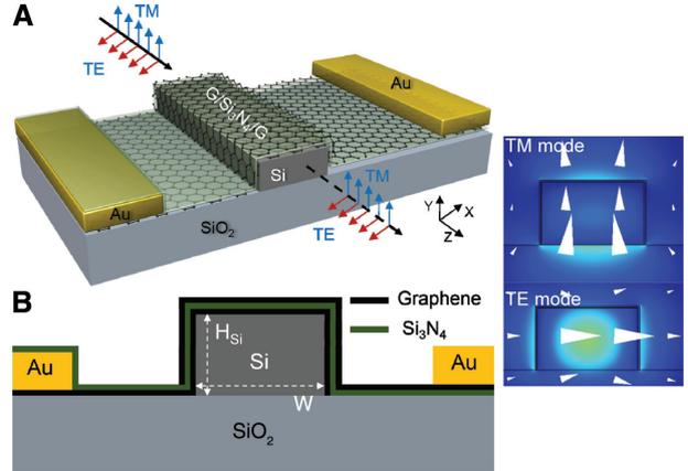
**Figure 2:** The structure of the polarization-insensitive optical modulator.
