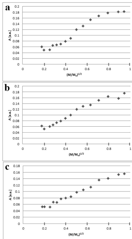
**Fig. 4.** The influence of microwave power ( $M/M_o$ ) on amplitude ( $A$ ) of the EPR line of *vaselinum flavum* sterilized at: (a) temperature 160°C for 120 min, (b) temperature 170°C for 60 min, and (c) temperature 180°C for 30 min. Data for the storage time after sterilization of 2 days.
