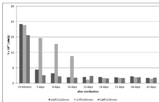
**Fig. 2.** The effect of storage time on free radical concentrations ( $N$ ) in *vaselinum flavum* sterilized at temperatures 160°C (120 min), 170°C (60 min), and 180°C (30 min).
