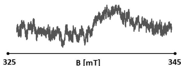
**Fig. 1.** The exemplary EPR spectrum of *vaselinum flavum* sterilized at temperature 160°C for 120 min. The measurement was done 20 min after sterilization with a microwave power of 2.2 mW.
