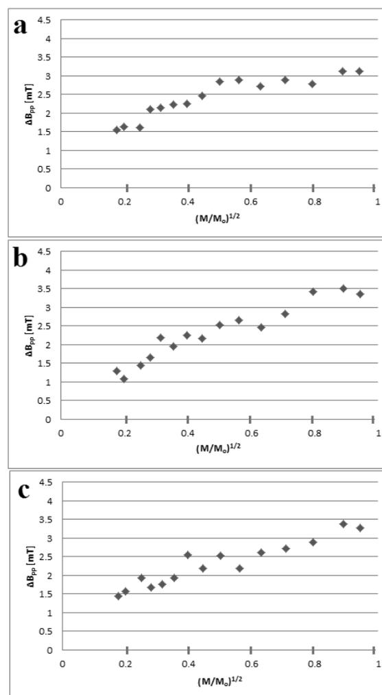
**Fig. 6.** The influence of microwave power ( $M/M_0$ ) on linewidth ( $\Delta B_{pp}$ ) of the EPR line of *vaselinum flavum* sterilized at: (a) temperature 160°C for 120 min, (b) temperature 170°C for 60 min, and (c) temperature 180°C for 30 min. Data for the storage time 40 days after sterilization.
