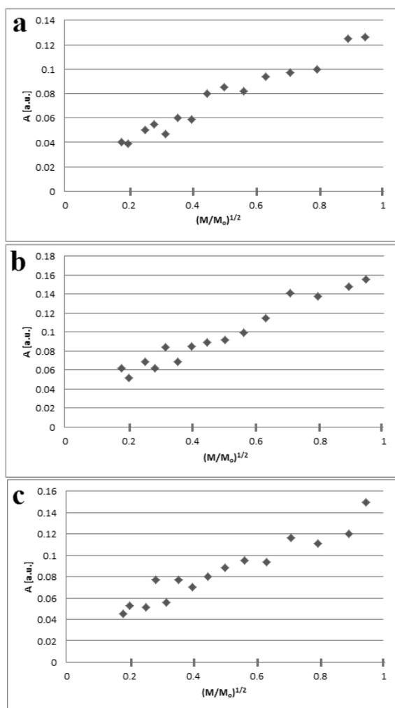
**Fig. 5.** The influence of microwave power ( $M/M_0$ ) on amplitude ( $A$ ) of the EPR line of *vaselinum flavum* sterilized at: (a) temperature 160°C for 120 min, (b) temperature 170°C for 60 min, and (c) temperature 180°C for 30 min. Data for the storage time 40 days after sterilization.
