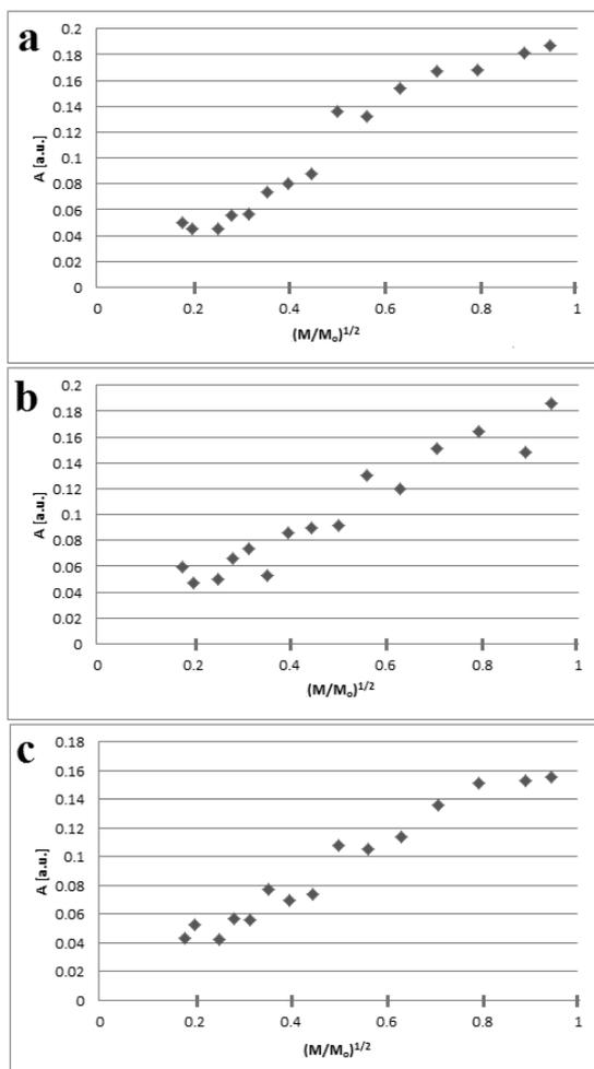
**Fig. 3.** The influence of microwave power ( $M/M_o$ ) on amplitude ( $A$ ) of the EPR line of *vaselinum flavum* sterilized at: (a) temperature 160°C for 120 min, (b) temperature 170°C for 60 min, and (c) temperature 180°C for 30 min. Data for the storage time after sterilization of 15 min.
