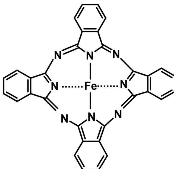
**Fig. 1** Molecular structure of iron phthalocyanine.
