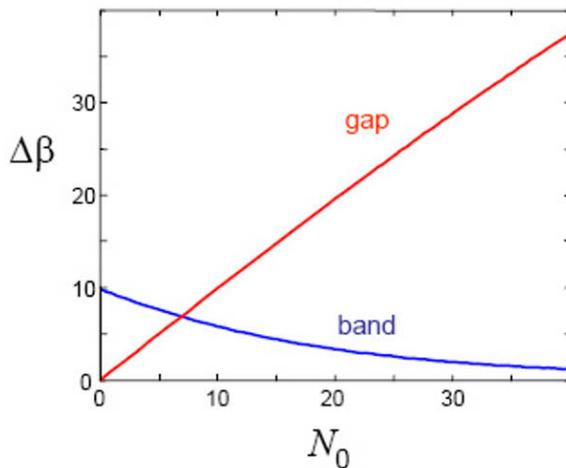
**Figure 3.** Width of the first band and of the first gap depending on the strength of the sinusoidal potential.
