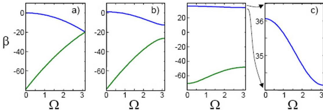
**Figure 2.** Band structures of particles in a sinusoidal potential of varying depth a)  $N_0=0$  (free particle), b)  $N_0 = N_c=6.9$ , c)  $N_0 = N_d=31$  (the first band is magnified to illustrate its cosine-like structure).
