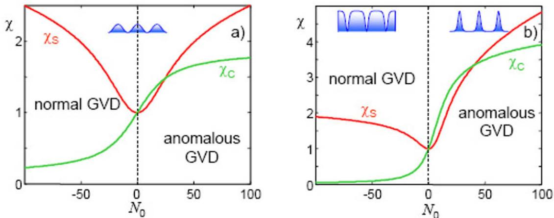
**Figure 7.** Effective nonlinear self-phase modulation of the signal wave  $\chi_s$  and the strength of its interaction with the lattice  $\chi_c$  for a sinusoidal (a) and a sech-like lattice (b) for normal ( $N_0 < 0$ ) and anomalous ( $N_0 > 0$ ) GVD at the signal wavelength.
