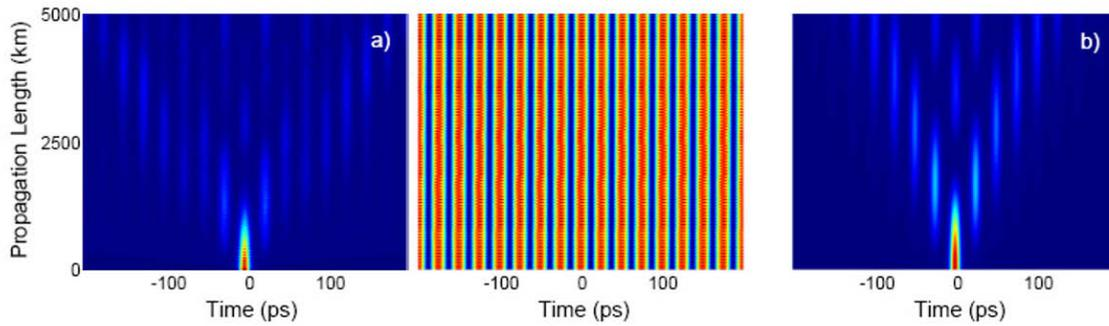
**Figure 6.** Discrete temporal diffraction in a sinusoidal lattice (parameters in the text) a) signal (left) and writing wave (right) are both subject to nonlinear action, b) signal wave for a fixed periodic potential.
