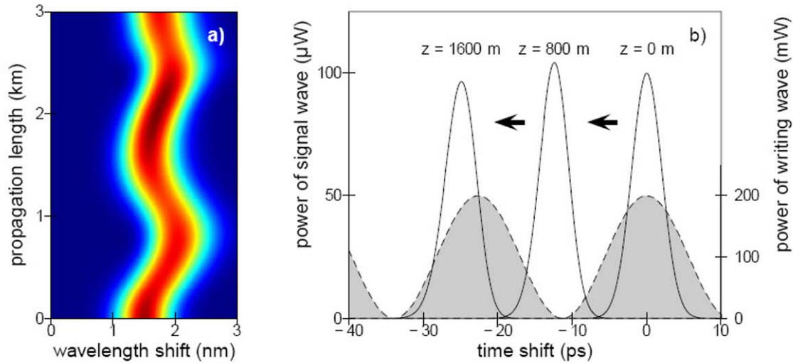
**Figure 8.** Bloch oscillations performed by a signal pulse in the spectral domain (a) correspond to a periodic interaction between signal pulse and writing wave in the temporal domain (b) (full line: signal pulses, gray area: writing wave).
