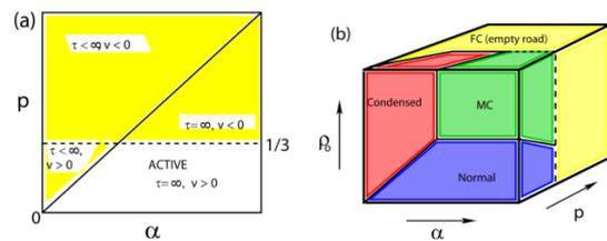
**Figure 2.** (a) A MF-based phase diagram of  $(p, \alpha)$  at constant  $\rho_0$ , where the type of lines indicates first order (dashed line) and second order (solid line). (b) The extended 3D phase diagram of the parking garage model with nonlocal hopping.
