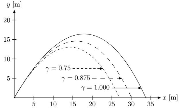
**Figure 1.** Projectile trajectories obtained from (14) and (16) for different values of  $\gamma$ ,  $v_0 = 22 \text{ m/s}$ ,  $g = 9.81 \text{ m/s}^2$ ,  $k = 0.1 \text{ s}^{-1}$  and angle  $\theta = \pi/3$ . The trajectories obtained in the fractional case, never exceed the ordinary ones  $\gamma = 1$ .
